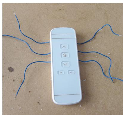
A small blob of thermocol on the wires makes sure that the printed circuit board does not com under stress when handling the wires, I can now control the sunscreen up, down and stop by touching the appropriate wires.
