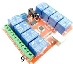
Connect the wires to the relays so that, when a relay is closed, a button is pushed, and when a relay opens, the button is released. I connected the down button to relay 1, stop to relay 2 and up to relay 3.
